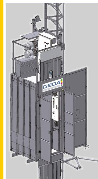
**GEDA SH 1000** Load capacity 1000 kg Car size 1100 x 1680 mm Lifting speed up to 60 m/min Lifting height 200 m
